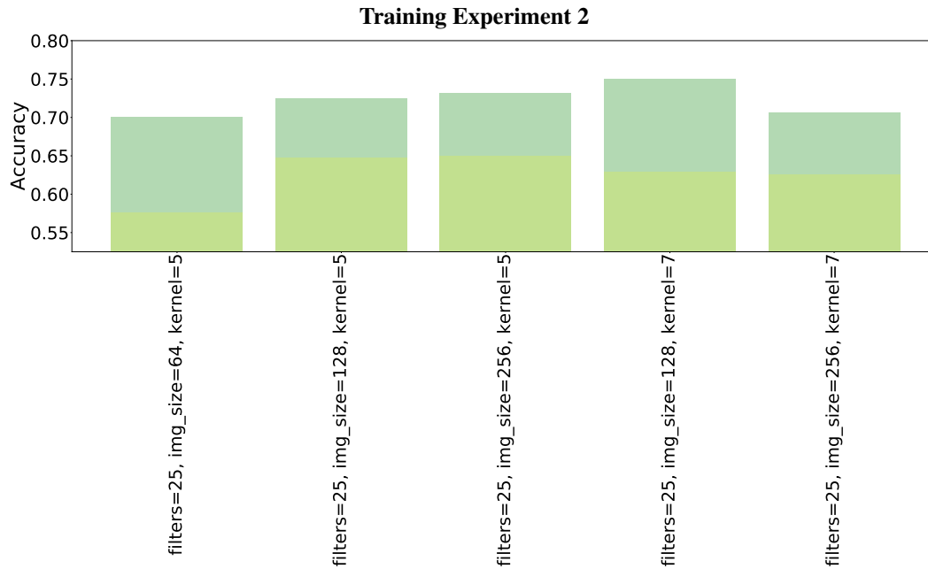
Figure 4: The effect of kernel size and image resolution on training. The lighter, lower mark, in each bar was best out of a 7 epoch moving average, the higher mark is best out of all epochs. The accuracy score is, as in figure 3, the weighted average we’re also using in the Kaggle test. Learning rate was 0.0001 across tests.
