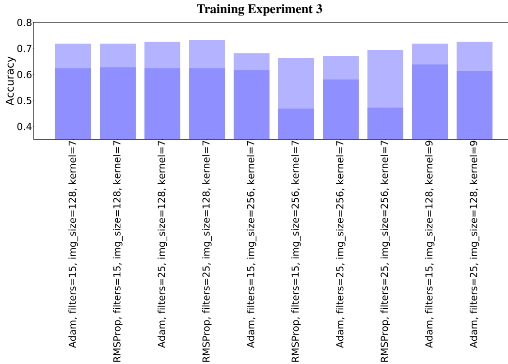
Figure 5: Experimentation with different optimizers, kernel size, image size and filters. The lighter lower mark in each bar was best out of a 7 epoch moving average, the higher mark is best out of all epochs. The accuracy score is, as in figure 3, the weighted average we're also using in the Kaggle test. Learning rate was 0.0001 across tests.
